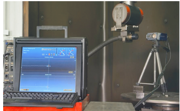
Figure 5 - Shotmeter system on a PROGRESSIVE CNC shot peen machine.
