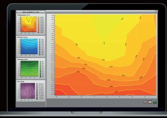
Correlates velocity and temperature with particle size for optimized spray parameters.
